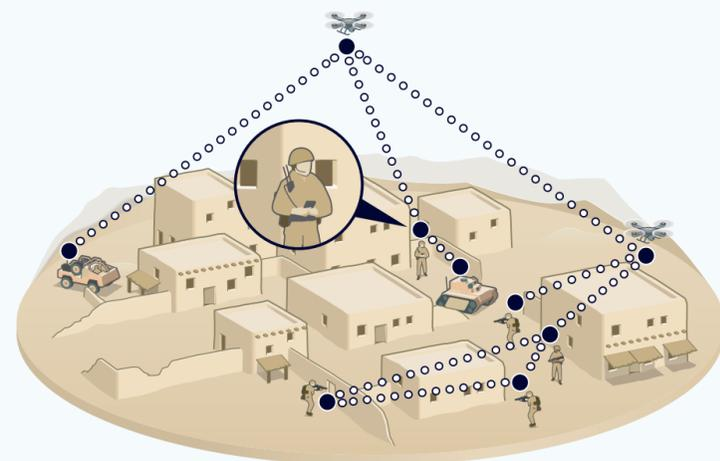
Enhanced situational awareness means better decision-making. Enhanced soldier-to-soldier communication means safer and more efficient mission execution. The SDR-H, powered by DTC's unique mission-critical Tactical COFDM Mesh waveforms, delivers high bandwidth Full Motion Video (FMV) from helmet and body worn cameras, low latency full-duplex voice throughout the team and supports the sharing of critical mission data on the ground where it is needed.
