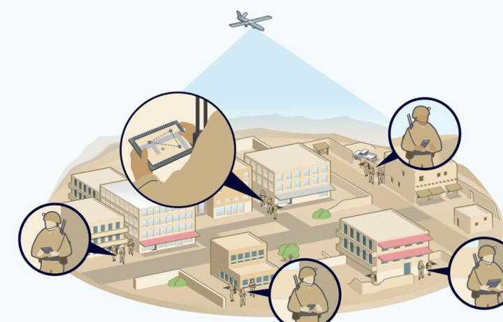
Direct video downlink from UAV platforms can provide unrivalled situational awareness on the battlefield, as well as close-in intelligence on targets and opposing forces. The SDR-H can operate in a "receive only" COFDM mode, using industry standard DVB-T or DTC proprietary narrowband
