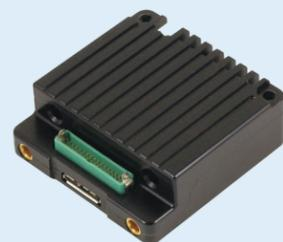
The SDR-C offers 2x100mW output in a tiny “Concealment” form factor, ideally suited for integration into small drones or other size/weight critical applications.
