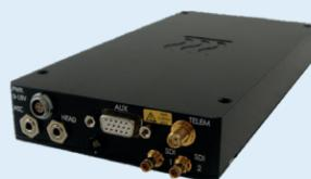
The SDR2x2W-P is a 2x2 watt MiMo Mesh radio in a practical enclosure suitable for desktop use or platform integration and incorporating industry-standard interface connection.
