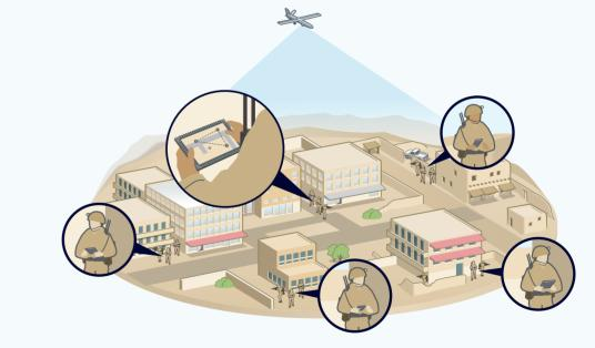
Direct video downlink from UAV platforms can provide unrivalled situational awareness on the battlefield, as well as close-in intelligence on targets and opposing forces. The SDR-H can operate in a "receive only" COFDM mode, using industry standard DVB-T or DTC proprietary narrowband COFDM waveforms to provide a low latency "one-to-many" downlink surveillance capability. In addition, the SDR-H IP Video straming capability can stream directly to existing tablets and PC' s.
